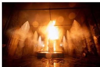
Marioff HI-FOG® high pressure water mist fire protection system with an electric pump unit has received an extended FM Approval to provide fire protection for combustion turbines and machinery with enclosures up to 2300m<sup>3</sup>, nearly doubling the amount of space covered.
